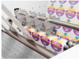
PRECISION SLITTING SYSTEM Utilizing rotary slitting mode which can install max.15 blades. High speed with 60m per minute takes place of traditional slitting equipment completely.
