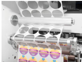
THE WASTE REMOVING SYSTEM The precision machinery design can control the roller rotating uniformly, avoid removing waste discontinuously due to unstable pressure and keep finished labels clean.
