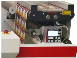
HIGH PRECISIONS FEEDING SYSTEM Utilizing the ultrasonic web-guide system, it makes the feeding perfectly.
